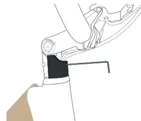
Adjusting the position, use a 2.5mm Allen wrench to secure the wire splitter cover.
