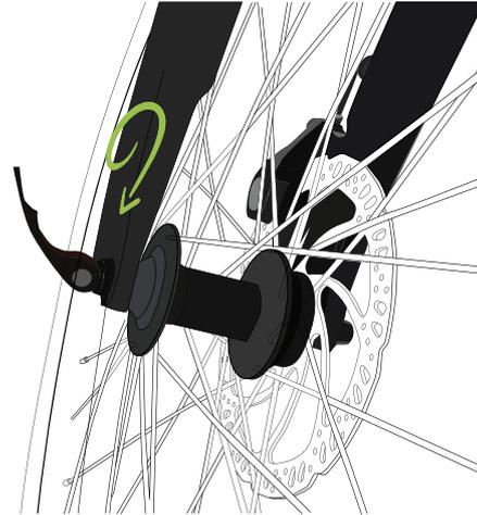
After tightening the axle, press the lever to lock it.
